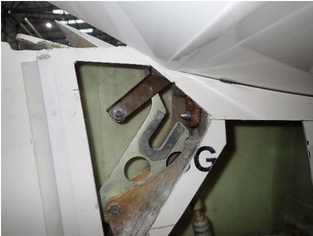
Disconnected elevator control
